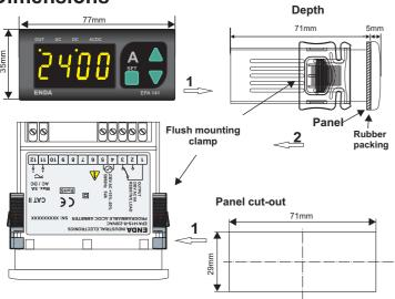
For removing mounting clamps:
