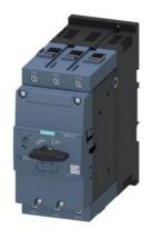
Circuit breaker size S3 for motor protection, CLASS 10 A-release 36...50 A N-release 650 A screw terminal Standard switching capacity
