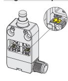
Articles with contact block C11, C02, C12, C22 are characterised by electrical contacts with a "V" design. This configuration reduces the possibility of error during operation and guarantees even more reliable contact switching, thanks to the contact points doubled compared to the flat-shaped contacts and the self-cleaning action of the contact. In the version with snap action contact, these articles are particularly suitable for use in the railway sector.
