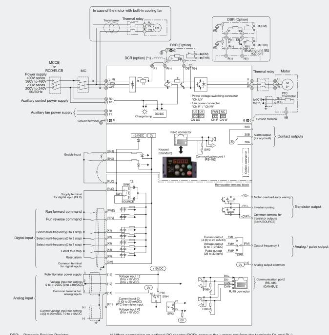
DBR: Dynamic Braking Resister DCR: DC reactor
