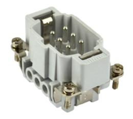
Male insert, JNE series, screw terminal connection, 6 poles + PE, 16 A 500 V 6 kV 3, size "44.27", with plate
