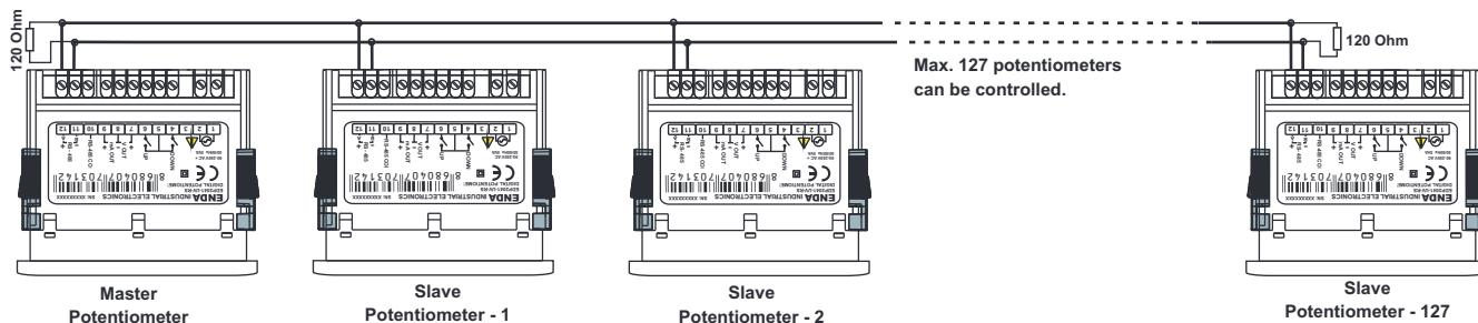
Max. 127 potentiometers can be controlled.
