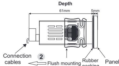
To remove the device from panel :
