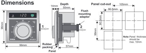
For removing mounting clamps: Push out the flush-mounting clamp in direction 1 as shown in the figure above. Then, pull out the clamp in direction 2. If there is no 60mm free space at back side of the device, it would be difficult to remove it
