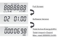
After the self-checking program, the meter display will show the total active energy (kWh)
