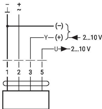
Override control (frost protection circuit)
